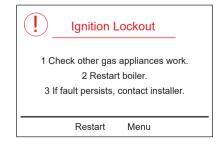
To restart the boiler, press Restart. The boiler will repeat the ignition sequence. If the boiler still fails to light consult a Registered Gas Installer.
