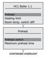
i. Preheat - Preheat can be enabled for a heating circuit and a maximum time can be set.
