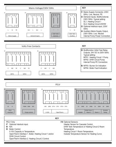
\*Note: The items grayed out are not standard and are connections provided by the relevant option kits.
