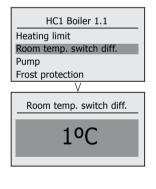
iv. Pump - The heating circuit pump overrun time can be set here. If the heating circuit pump is controlled by 0-10V then additional speed parameters can be set.
