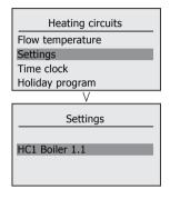
i. Preheat - Preheat can be enabled for a heating circuit and a maximum time can be set.
