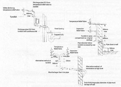
Note: The discharge will consist of scalding water and steam. Asphalt, roofing felt and nonmetallic rainwater goods may be damaged by such discharges.
