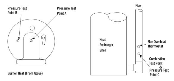
Fig 6.1.1 Pressure Test Point Locations
