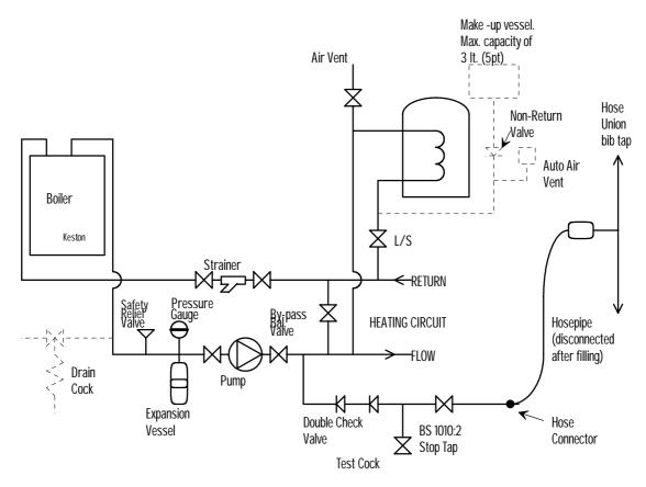
Figure 2.7.2 : Sealed System Diagram
