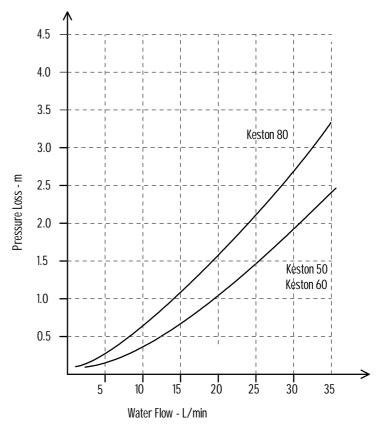
Figure 2.7.7: Pressure Loss Graph
