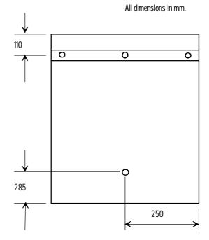
Figure 3.1 Wall Mounting Fixing Locations
